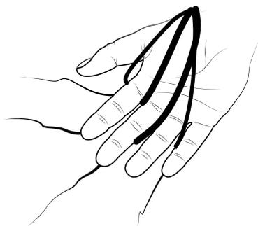
2 Start at the leading edge and sort the bridle lines. Then connect your grey front lines with a larkshead at the end of the bridle line as shown in the picture. Attach your colored backlines with a larkshead with the colored pigtail to the tip of the kite.
