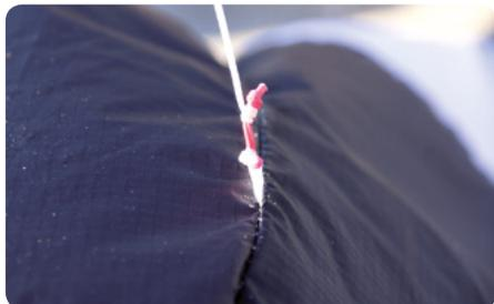
The "Little Connection Line" (LCL) allows you to quickly exchange a bridle line and also works as a predetermined overload weak-point that prevents the canopy from getting damaged. Should an LCL break, replace it with a new LCL of the same colour (same breaking strength).
