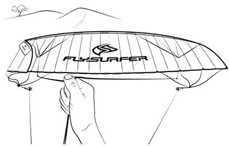
**7** When the bridle is sorted out, lay the front lines to the inside and the steering lines to the outside. If not, follow the tips on the "Sorting out the bridle" chapter.
