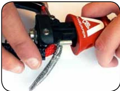
Pay attention that the sleeve of the Chicken Loop goes through the Unhooked Line. Next, let the red release sleeve spring downward.
