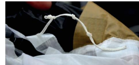
The PMAs are small knotted lines with two settings which are stitched into the airfoil on the top and bottom. Thereby the airfoil can be directly adjusted as illustrated below.
