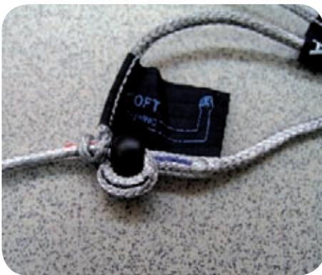
Adjusting the steering forces on the PULSE 2 is almost the same as it is with the SPEED 2. The difference is that you can adjust the steering forces continuously by just moving the ball /metal ring up or down on the WAC Line towards Hard- or Soft-Steering. Coloured markings on the line help with the orientation. Pay attention to equally position the ball on both sides!
