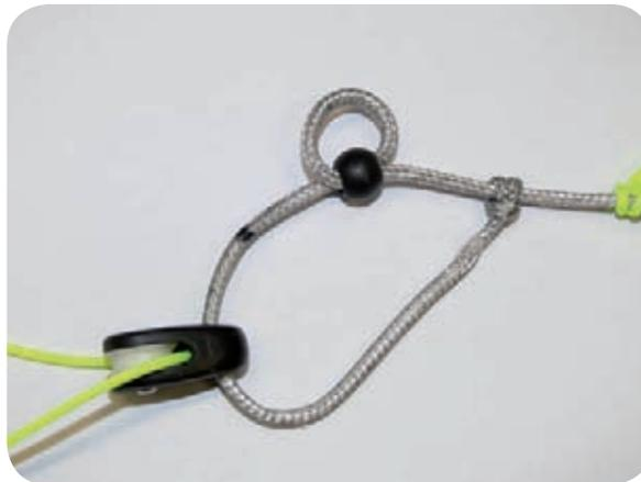
Move the position of the plastic ball by loosening the line which is guided through the ball. Depending on whether the lines should become shorter or larger, move the ball in the desired direction and tighten it again.
