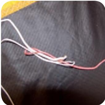
Because this line runs through a ring, there is more wear and tear on the line than on the Bridle Lines. FLYSURFER recommends paying particular attention to the Tip-Sparepartline during any Kite check. Through the wear and tear, the Line will begin to exhibit alterations and/or discoloration (the structure breaks down) and will ultimately shorten.
