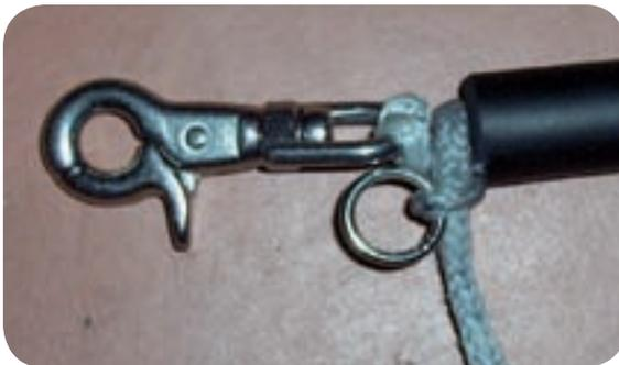
Then hook, like at a pure depower-loop leash, the shackle into the white loop on the right side of the depower loop (Half-Force-Line).
