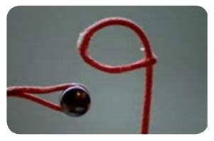
In order to connect a line put one ELC in one noose of the two ends to be connected. With the other loop create a loose larks-head knot. Now insert the ELC through the loop of the second noose (not through the larks-head knot itself) and tighten the larks-head knot.
