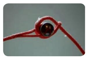
It is important that the lines all run in the groove of the ELC. Compare the result with the picture and check if the connection is tight.
