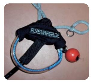
Create a loop with the end of the FLS or FDS (depending on the system set up. For this purpose you must put the line through the spliced loop at its end. (Don't put the line through the ring! This might release without intention.)
