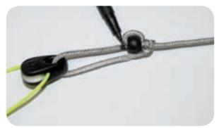
It's useful to mark the position of plastic ball before with a pin, so you can always restore the beginning position, and see exactly, how much you moved the ball. The adjustment of the B and C line works as follows:
