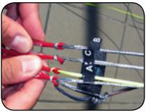
Remark: it is practical to mark the starting position with a pen. This way you can establish your starting point again and see exactly how much you have adjusted. Start adjusting the C level as this will move the B level automatcally half the way!
