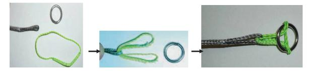
Pull the grey FDS-Endline through the bar and the center of the chickenloop, and connect the yellow weakpointline and the ring.
