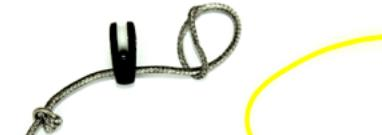
**5** Put the pulley through the loop.
