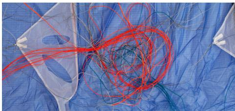
3 Lightly tension up the bridle again to check it. If necessary, repeat the last step till the left and right bridles are separated.
