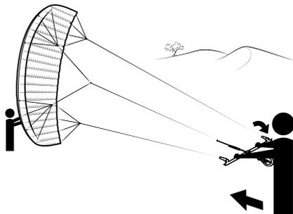
❺ Secure the kite as described in "Securing the Kite".
