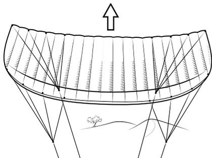
**3** When the kite is at least one wingspan above the ground, let go of one of the leader lines. Make sure you keep hold of the other one and the bar is in the right position.
