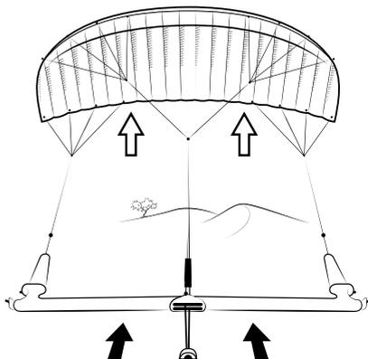
*Tip: The reverse launch is the recommended relaunch method when kiting on solid terrain. This minimises potential damage from abrasion.*
