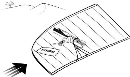
**4** Lay the bridle lines in between the folded kite.
