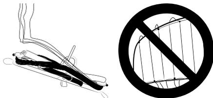
**4** Start at the leading edge holding up the front lines to visually check the bridle step by step.
