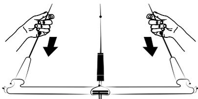
**2** Pull in both leader-lines as far towards yourself as possible to reverse the kite off the ground. Strong pulls or pumping the lines may help in light winds. If the kite does not release from the ground, grab the leader lines higher up.
