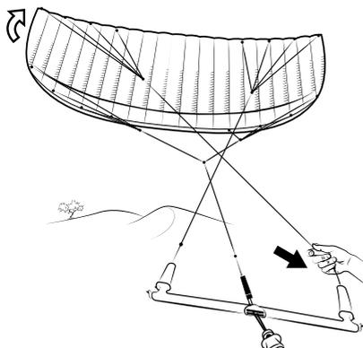
**4** The kite will now spin around. As soon as the leading edge of the kite points up let go of the remaining leader line and put your hand back on the bar. Depower the kite till its back in the sky towards the zenith.
