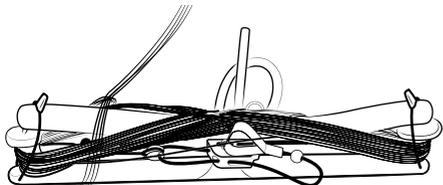
**2** Fold the kite in half along the middle (tip on tip) and make sure that the bridle is inside both halves. Also make sure that there are no bridle lines over the outside skin.
