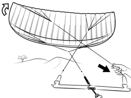
*If the kite does not lift up and peel to one side when pulling the leader line, try pulling the opposite leader instead. If this still does not work, then use the reverse launch method.*
