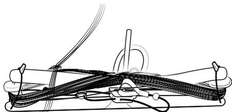
2 If necessary, undo loops, knots, or balls of balls. Most loops can be loosened by pushing the bar through along the line.
