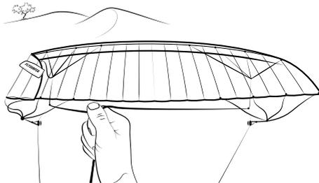
**5** When the bridle is sorted out, lay the front lines to the inside and the steering lines to the outside. If not, follow the tips on the "Sorting out the bridle" chapter.
