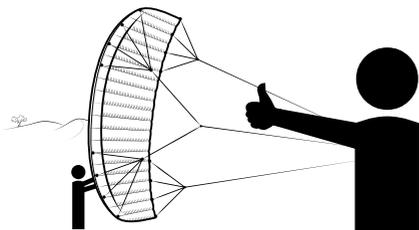
② Put the flying lines under tension so that the kite rises slowly. Take another step to windward to release the weight from the trailing edge of the kite.
