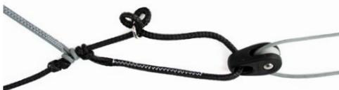
**Tip:** The mixer is a 2:1 pulley system. If you want to change the B-Level by one centimeter, you will need to move the ring by two centimeters.
