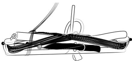
2 Undo any loops, knots or bunches that may have formed. If the bridle is tangled, lines from one side of the bridle may be running through the lines on the other side. Stick the bar along these lines through the bridle.
