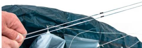
5 If this is not the case, you just have to move the metal ring of the mixer (C-Level) until all 3 knots are at the same level.
