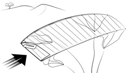
2 Pre-inflate the kite at least half way, for more control during the launch. The kite should be positioned 15-30° downwind of you when you slowly tension the lines for launch.
