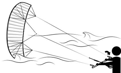
❷ The excessive water/dirt should now flow out of the tip until it is ready to be launched again.
