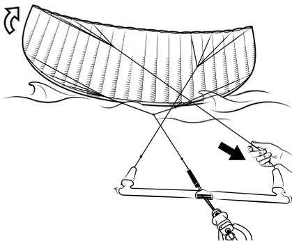
*If the kite does not lift up and peel to one side when pulling the leader line, try pulling the opposite leader instead. If this still does not work, then use the reverse launch method.*
