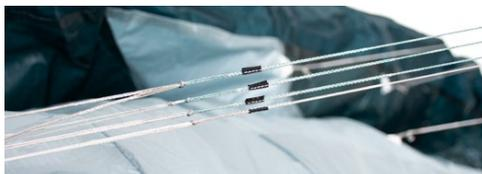
7 If this is not the case, you just have to move the metal ring of the mixer (B-Level) until all 4 knots are at the same level.
