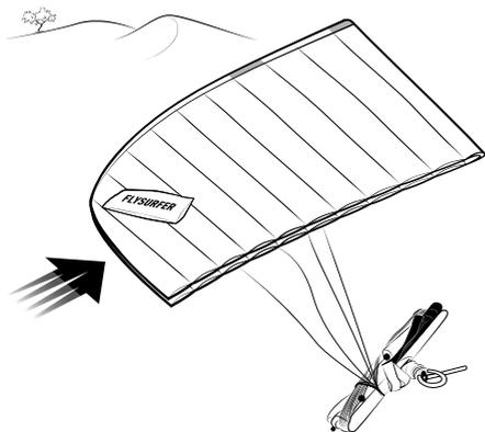
**2** Open the kite and if necessary, close the deflate valves. Unroll the lines from your bar whilst walking away from the kite.
