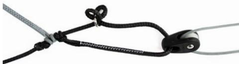
*Tip: The mixer is basically a 2:1 pulley system. If you want to change the B-Level by one centimeter, you will need to move the ring by two centimeters.*
