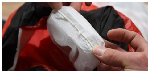
**3** Adjust the PMA by moving the larks-head-knot.
