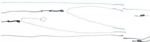
4 When exchanging a pulley (after 250h of use) concentration is needed. First make a larks head at the end of the line.
