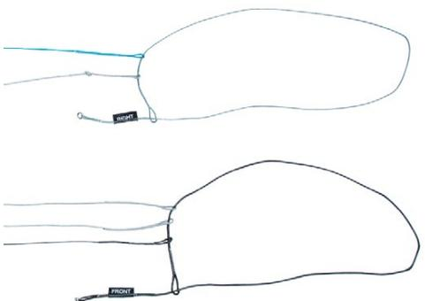
9 Reconnect the flying lines again, and then repeat the same procedure on the other side. Pull all knots tight and check the bridle carefully.
