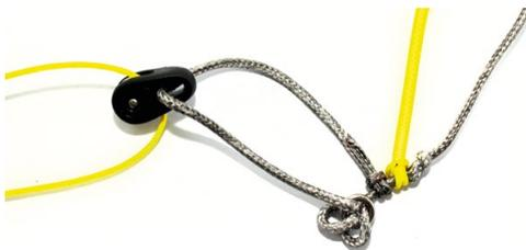
**Tip:** The mixer is basically a 2:1 pulley system. If you want to change the B-Level by one centimeter, you will need to move the ring by two centimeters.
