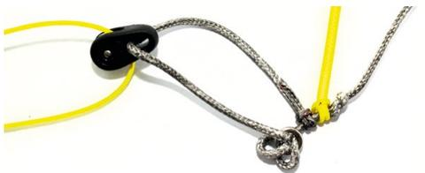
**Tip:** The mixer is basically a 2:1 pulley system. If you want to change the B-Level by one centimeter, you will need to move the ring by two centimeters.
