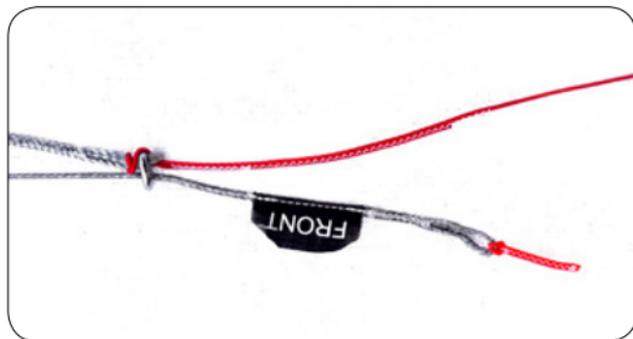
7. Using a larks head knot, connect the red FDS-extension from point 3 to the FDS-flyingline. This connection allows you to change the control bar and flying lines to another size SPEED5 with FDS System.
