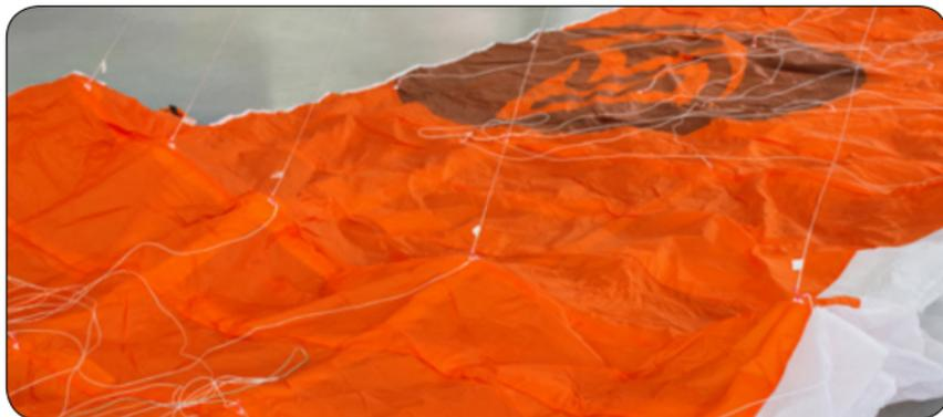
3. Loop the FDS-extension through the end of all five FDS-toplines. Make sure that the FDS-toplines are lined up one after the other. Finally tighten this connection.
