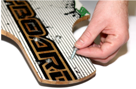
1. Insert the screws into drilled whole
