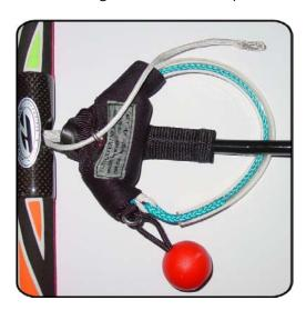
5 Finally, connect the big steel ring to the end of the FDS-Endline, then the ring through the sleeve of the line, this way:
