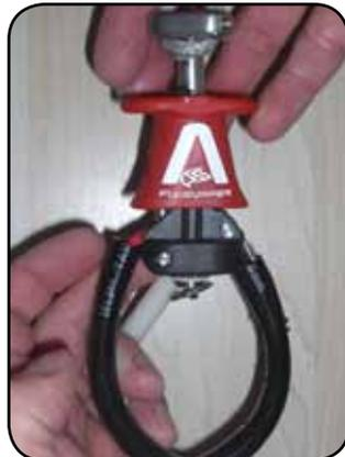
To Reset the Loop push the end of the pin through the Red loop and push the pin up toward the cover. Let the cover go and let it slide back over the pin.
