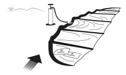
2 Look to see if the check valve is closed. If it is not, then press the pin – this should then visibly stand out of the valve.
