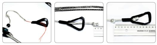
11. Remount the front lines to the depower leader line using a larks head knot. Guide the safety-endline through the steel rings and then through the bar eyelet.
