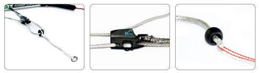
10. Make a loose knot on the adjuster line and pull the adjuster line through the handle. Add a knot to the end of the line to fix the handle (tail length = 10 mm). Fasten the first knot at a position 20 mm behind the handle.
