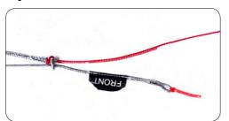
7. Using a larks head knot, connect the red FDSextension from point 3 to the FDS-flyingline. This connection allows you to change the control bar and flying lines to another size SPEED5 with FDS System.
