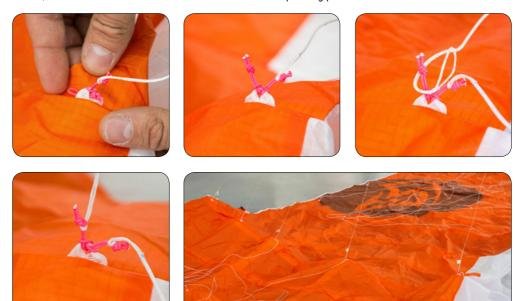
3. Loop the FDS-extension through the end of all five FDS-toplines. Make sure that the FDS-toplines are lined up one after the other. Finally thighten this connection.
