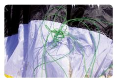
• If the bridle is tangled, lines from one side of the bridle may be running through the lines on the other side.
