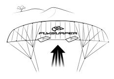
fill through the air intakes. Wait until the kite has been prefilled enough before launching.
