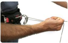
When you reach the bar, secure the endline to your harness hook. This is done by wrapping the side of the endline which is under tension two times around the harness hook and then the loose side one time in the opposite direction.
