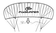
3 Secure the leader lines around a suitable object in a way that the back-lines stay "braked" and flying up of the kite again is not possible.
