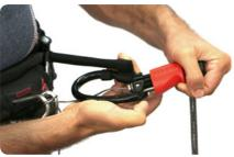
**(b)** Let the Chicken Loop go and unwrap the endline from the harness hook. Make sure you have a good grip on the endline as you hook in the Chicken Loop and secure it with the Chickenstick.
