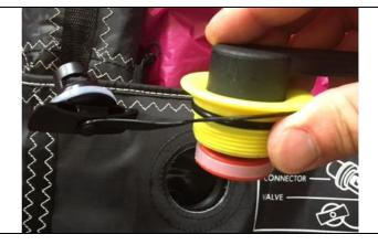
Screw the valve with the valve wrench clockwise into the basement.
